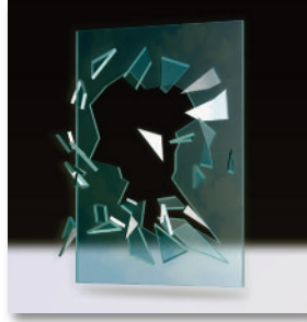
ANNEALED GLASS breaks easily, producing long, sharp splinters.
